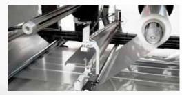
The tensioning unit ensures precise feeding even at the end of the reel.
