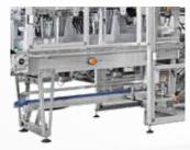
The pad/tray magazine, adjustable according to the dimensions of the blanks, is located under the channelling belt in order to be quickly refilled.
