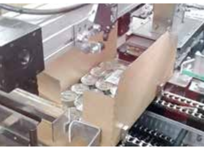
Pick&Place module with magnets.
