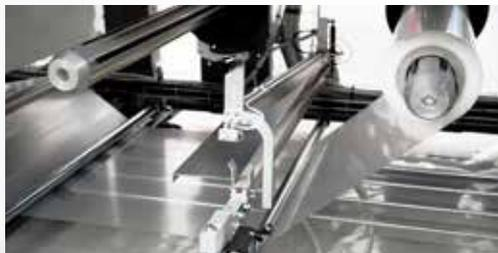
The tensioning unit ensures precise feeding even at the end of the reel.
