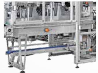
The pad/tray magazine, adjustable according to the dimensions of the blanks, is located under the channelling belt in order to be quickly refilled.
